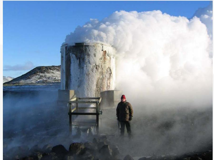
Discharging HT-well with separator at Hellisheiði
