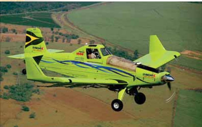
Airplane regularly produced to use pure hydrous ethanol (EMBRAER, 2008)
