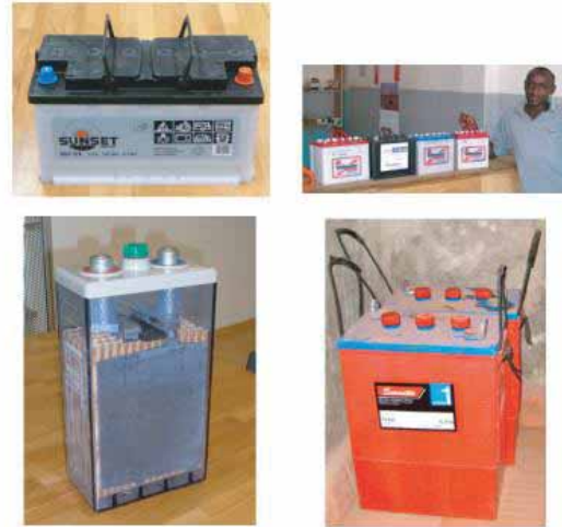
Figure 4.9 Types of battery; Sunset flat plate solar battery (top left); local Kenyan SLI batteries, not generally recommended but often the only option (top right); Hoppecke 2 volt cell, flooded, tubular plates, deep cycle, recommended for larger systems (bottom left); Surette 6 volt batteries, deep cycle (bottom right)
