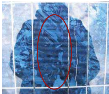
Broken cell, similar behavior as a shaded cell
