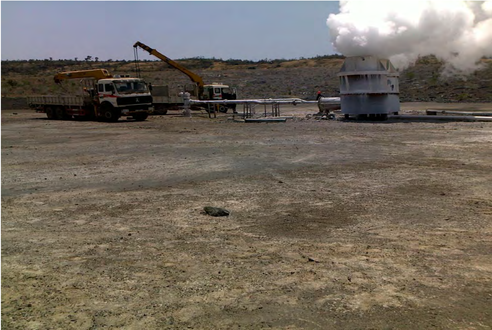
Plate 3: Reservoir engineers undertaking well head testing at Menengai Well No. 1
