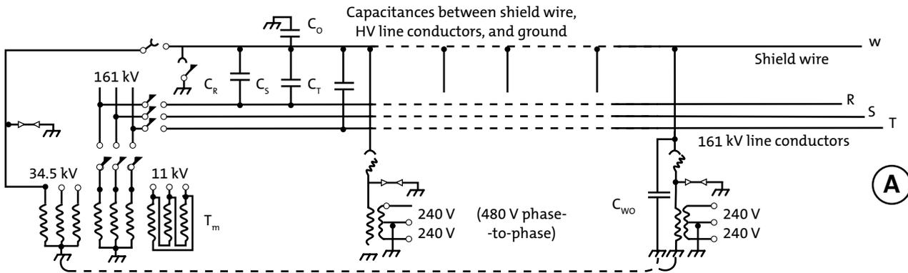
In shield wire systems, these shield wires are insulated from the tower and ground and provide a conductor for transmission of electricity. They are energized at MV (20–34.5 kV) from a HV/MV transformer stationed at one end of the HV line. MV/LV transformers are then added along the HV line to supply the loads. There are four main systems within SWS. They are:
