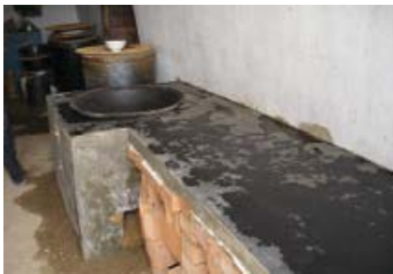
Figure 3.3b: Improved Biomass Stove-bed Device, Inner Mongolia
