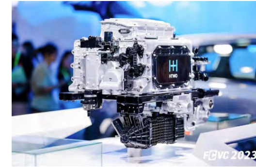
Hyundai Modern fuel cell stack
